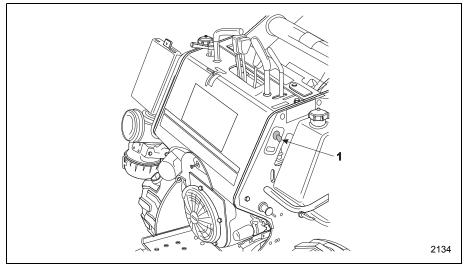
Figure 3-9 Engine Keyswitch
